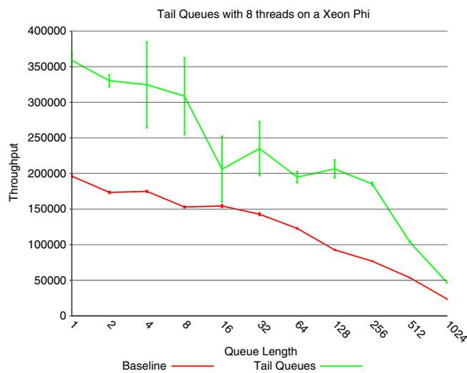
FIGURE 6 Tail queues prototype using eight threads on a KNC
