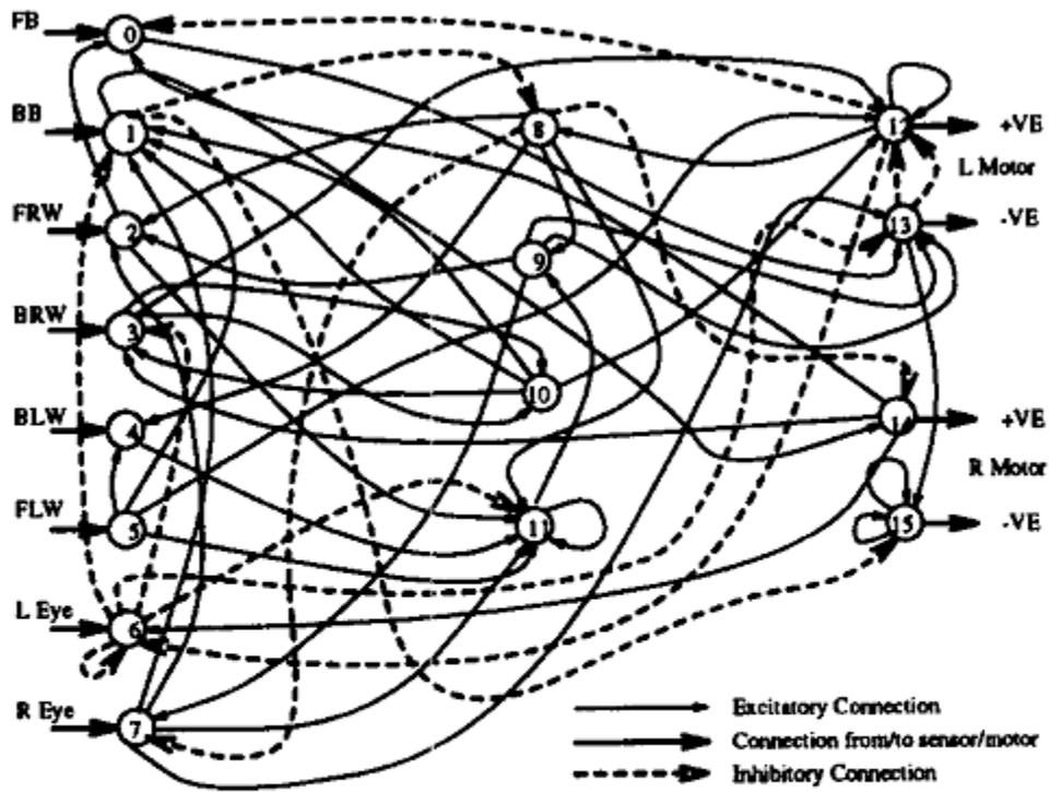
Fig. 11. Full C2 control network. The left-hand column are units originally designated as input units: FB=Front Bumper; BB=Back Bumper; FRW=Front Right Whisker; BRW=Back Right Whisker; BLW=Back Left Whisker; FLW=Front Left Whisker. Right-hand column shows output units, which are paired and differenced to give two motor signals in the range  $[-1, 1]$  from four “neuron” outputs in the range  $[0, 1]$ . Centre column shows “hidden units”.
